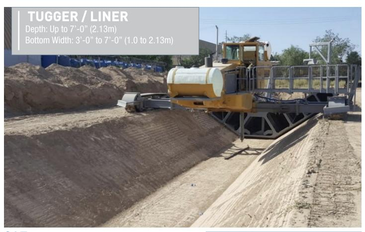
**G&Z** produces the highest quality, lowest operating cost Canal Liners available on the market today. Combining years of field and manufacturing experience, and utilization of the latest technology, makes Eagle Canal Liners the most cost-effective way to increase productivity and profitability.
